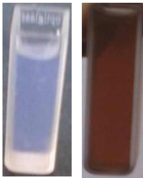
Fig. 1. Photograph of silver nitrate solution (a) Before reduction to nanoparticles (b) After nanoparticle formation
